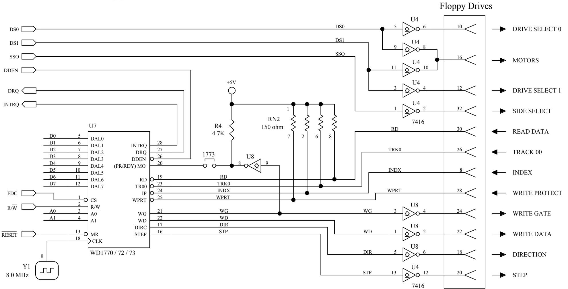
All odd numbered pins connect to GND.
