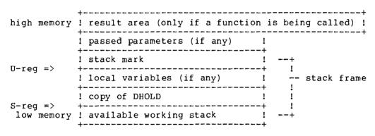
Figure 4. STACK CONTENTS DURING PROCEDURE EXECUTION.
