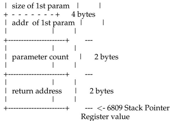
**Figure 9-1. Stack Frame Passed to Machine Language Procedures**
