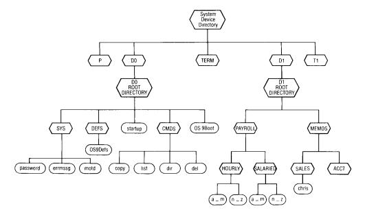
The disk in Drive 0 is the OS-9 System disk. Its root directory contains two files (startup and OS-9Boot) and three sub-directories (SYS, DEFS and CMDS). The sub-directories contain another level of files. All of these files are necessary to run OS-9.
