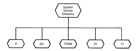
The P is the printer, D0 is the first disk drive, TERM is the keyboard/display, D1 is the second drive, and T1 is a terminal connected to the RS-232C serial port. (Even if you don't have the actual device, your directory still has the entry.)
