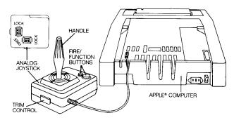
Analog Joystick for Apple® II, Ile and II Plus Home Computers CONNECTION: To connect the WICO Computer Command Apple® analog joystick, first remove the Apple® computer cover. Next, carefully insert the joystick plug into the 16-pin game I/O port and run the connector cord through the slot provided on the rear of the Apple® unit, as shown in diagram. Then replace the computer cover, and your joystick is ready for operation.
