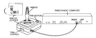
Analog Joystick for Radio Shack® TRS80® Color Computer CONNECTION: To connect the WICO Computer Command Radio Shack® analog joystick, simply plug the computer connection plug directly into the Color Computer joystick panel input. Your joystick is now ready for operation.
