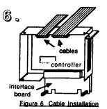
Install the 20 pin and 34 pin cables that will connect your controller to your hard drive. When you have correctly connected the cables to the controller, bend them up and over the top edge of the bottom cover.
