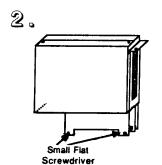
Figure 2 Top Cover Removal
