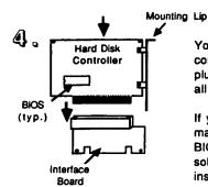
Your hard disk controller board plugs into the 62 pin connector on the interface board. Make sure that you plug the boards together "face up", so that you can see all of the parts that are mounted on each board.
