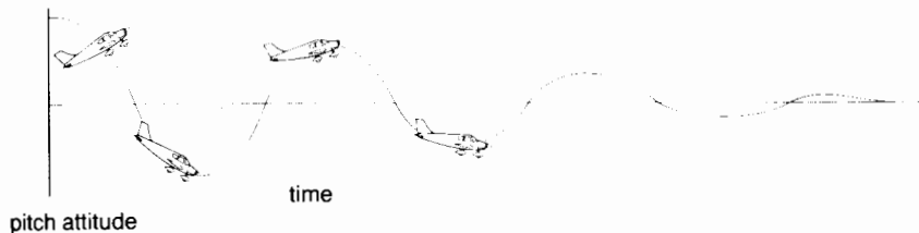
Figure 14. Positive Dynamic Pitch Stability
