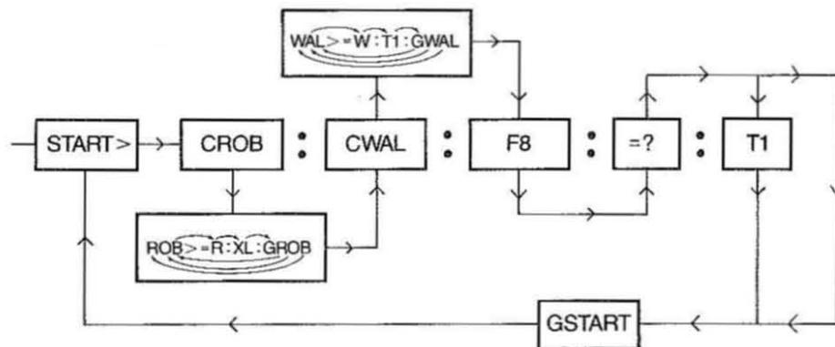
Figure 3. Flow chart of current routine for the left robot.
