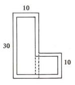
Add 30 by 10 by 1 Add 10 by 10 by 1 Subtract 29 by 9 by 1 Subtract 9 by 9.5 by 1 Subtract 9 by 0.5 by 1 Total volume = 49 Large Small Large inner Small inner The small dotted piece
