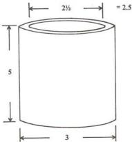
Calculate the outside measurement first. Make sure the total volume is set at zero and press ① for RECTANGULAR OR CYLINDRICAL?. Press ① for ADD OR SUBTRACT?. For DIAMETER?, type ③ and press ENTER. For HEIGHT?, type ③ and press ENTER. You then have the volume of the outside measurements of the ring, 21.18. However, you need to subtract the volume of the inside space to have the volume of the example object.
