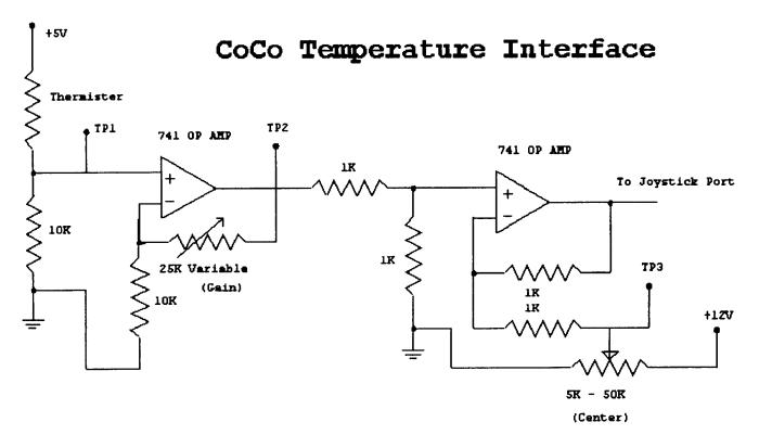
For Temperature sensing range of 50 to 114 degrees F
