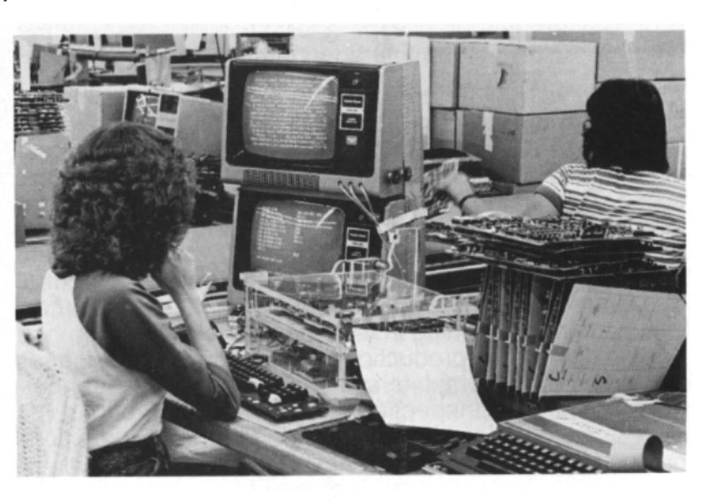
Burn-in, though it sounds like shades of the Inquisition, is simply a stress test for the board. All of memory is written to; the content of memory is verified for accuracy; and it is written to again. This goes on over and over for a full twenty-four hour period. If a chip is going to fail it will likely happen at this point.
