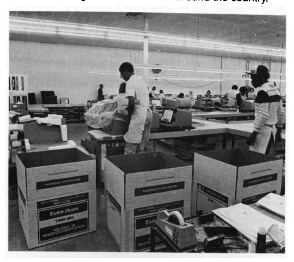
When the Model III arrives at the Regional Warehouse, it is pulled out of the box where it is put through another full system test. If the computer survives this system test it then goes for another twenty-four hour burn-in. Is there no end?
