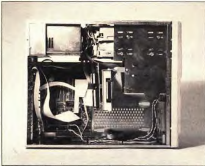
Photo 1: the TC9 case allows plenty of room for drives, controllers and the motherboard.
