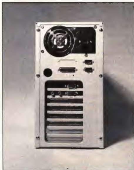
Photo 3: The connectors on the rear of the TC9 case are clearly labeled.
