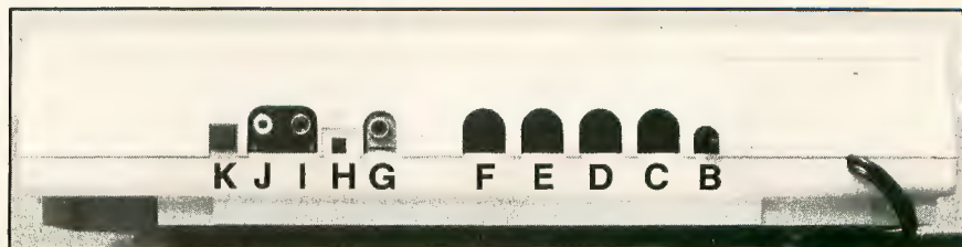
Right: The back of the Color Computer 3. All letter designations coincide with those in the circuit board view as well as those in the text.
