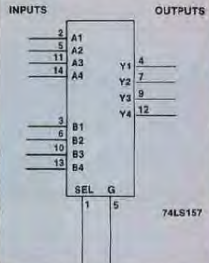
Figure 9 Read multiplexer type 74LS157 has eight lines in and four lines out. Two are used to multiplex a 16-line address bus.
