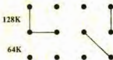
Jump Pin #1 to Pin #27 on EPROM
