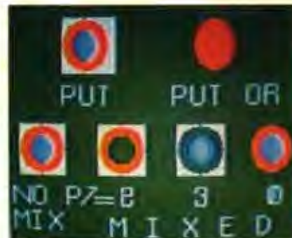
Picture 2: MIX option in PMODEs 1 and 3. Top using PUT. Bottom using Animatic with several MIX color combinations.
