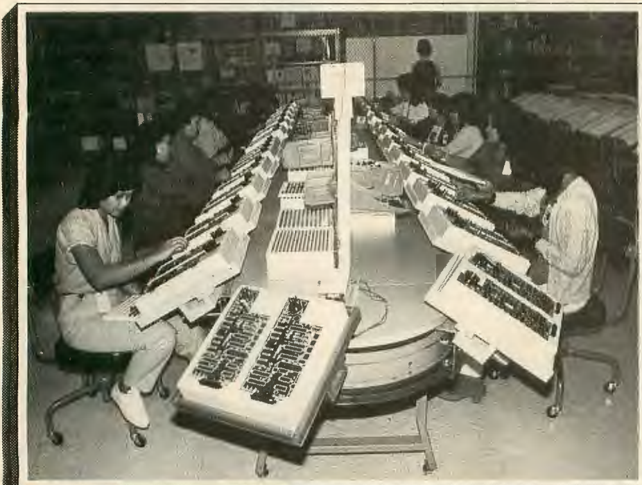
Each assembler handles one part to stuff on each board during a given cycle, a unique system here in the U.S.
