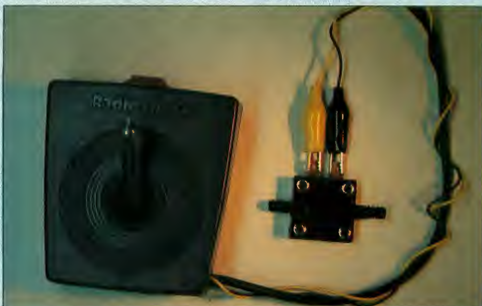
Puff/sip switch connected to the Color Computer 2 through a joystick.
