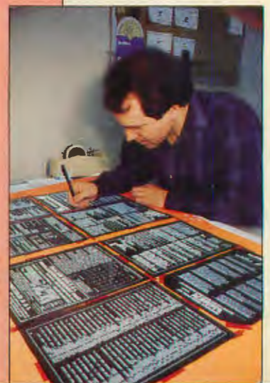
Cameraman John Pike makes plate-ready negatives from art boards of finished pages.
