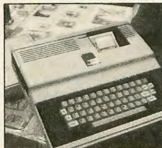
CoCo Max author Tim Jenison has customized a TDP-100 (a CoCo-clone, which Tandy no longer markets) by adding both a disk drive and black and white TV inside the case!
