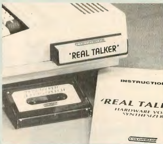
'Real Talker' is a full-featured electronic voice synthesizer unit built into a compact cartridge case. You simply plug it into the side of your computer.
