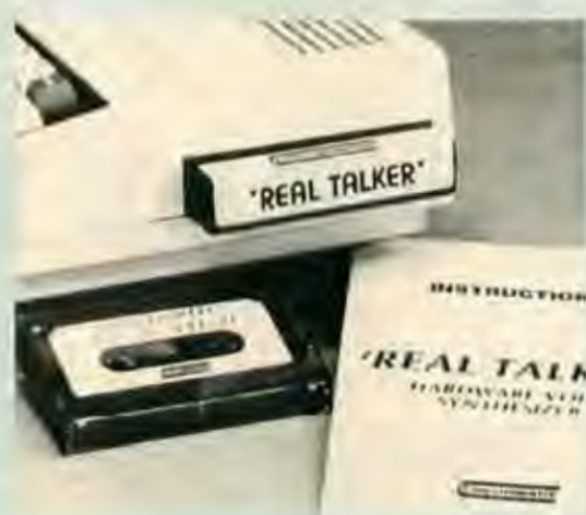
'Real Talker' is a full-featured electronic voice synthesizer unit built into a compact cartridge case. You simply plug it into the side of your computer.
