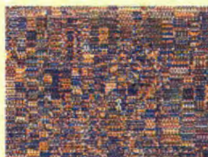
Figure 3: Encoded version of Figure 1 (Every byte of Figure 1 is XORed with corresponding byte of Figure 2)
