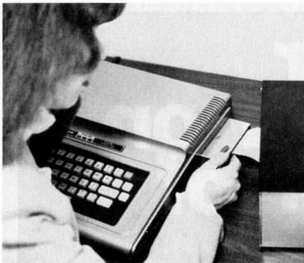
1. Here is Jeri plugging The Solution into the CoCo. Then she will move the main case up close to the CoCo. The cable is kept short to prevent noise and interference. The disk controller can be plugged into the side slot. The power supply plugs into a socket on the back of the case. All wires for the internal boards exit out the back of the case.
