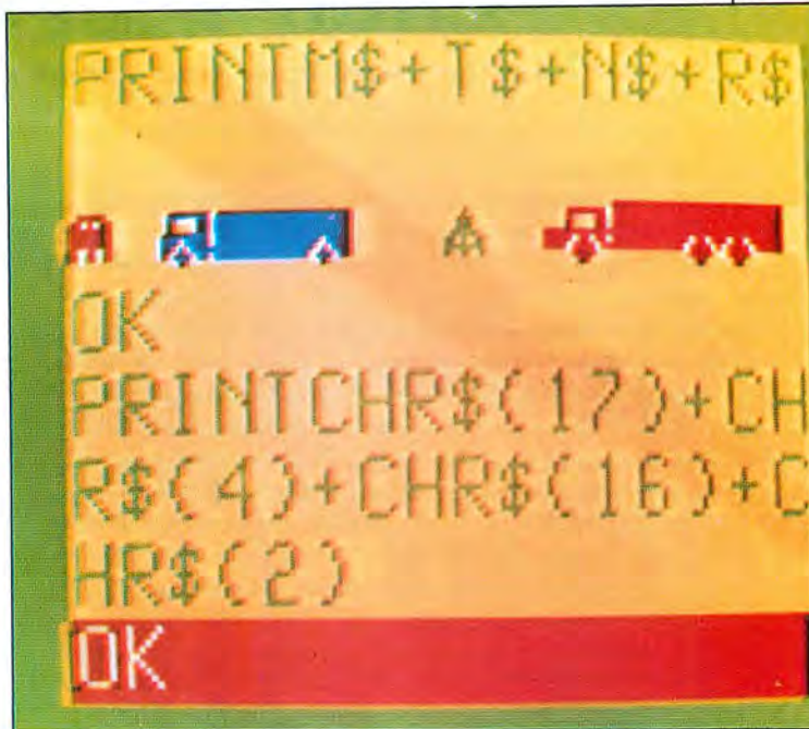
Photo 2. An example of Mul-T-Screen's ability to represent longer graphic characters and their colors and change the background color.
