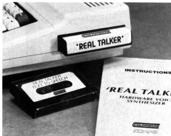
'Real Talker' is a full-featured electronic voice synthesizer unit built into a compact cartridge case. You simply plug it into the side of your computer.
