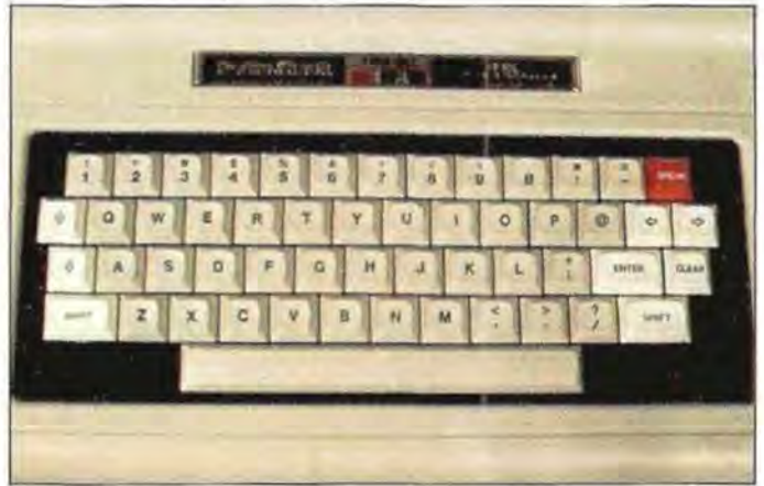
Photo 7. Radio Shack also improved the CoCo's keyboard. The keys are sculpted, giving the typist a better feel.
