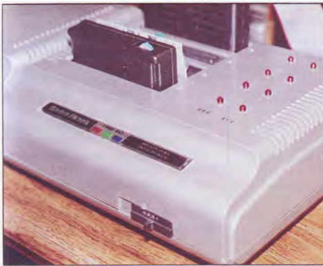
Photo 1. The MPI complete with on/off and slot-selection LEDs installed.
