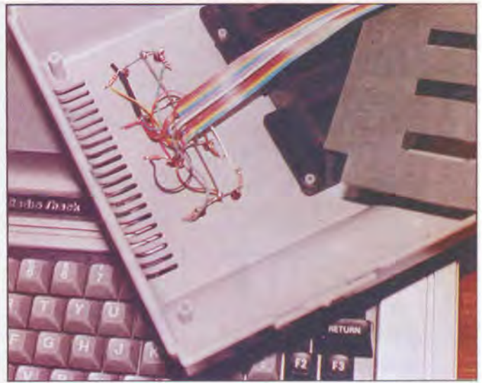
Photo 2. Here the internal LED wiring is displayed.
