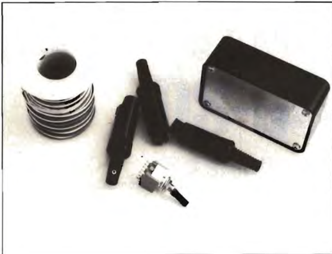
Photo 1. Parts Needed for the Switch Box
