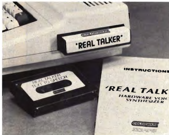
'Real Talker' is a full-featured electronic voice synthesizer unit built into a compact cartridge case. You simply plug it into the side of your computer.
