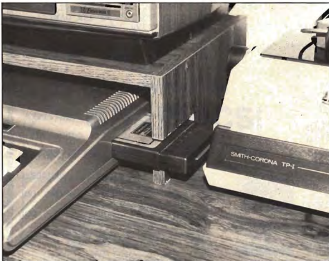
Photo 3. If your desk has a monitor stand, you'll probably have to modify it to accommodate ROM packs.
