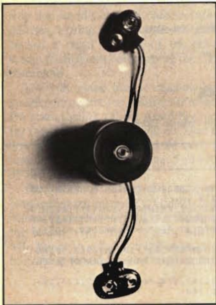
Photo 2. A simple circuit that allows one to borrow a toy, for computer games. Parts consist of two 9V battery snaps, a 1/8-inch jack, and a 35mm file container (improvise).
