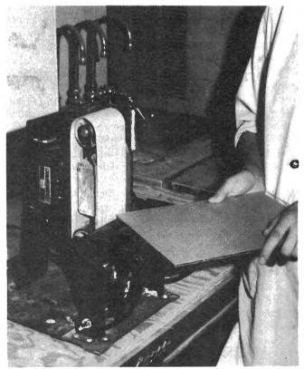
Figure 1: Sanding the edges of a plexiglass screen on a belt sander.
