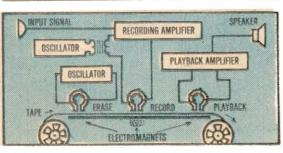
MAGNETIC RECORDING WAS INVENTED BY VALDEMAR POULSEN IN 1889. TAPE RECORDING WAS DEVELOPED IN THE LATE 1930'S. THIS DIAGRAM SHOWS HOW TAPE IS RECORDED.
