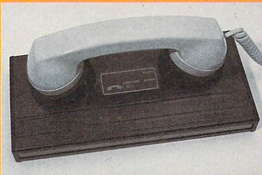
Acoustic-coupled modems like this Atari model grip the telephone handset with tightly fitting rubber cups to keep outside noises from interfering with communications.
