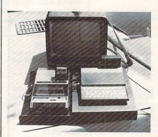
Car Comp secures a Timex/Sinclair and cassette deck as well as allowing power to be drawn from a standard auto cigarette-lighter outlet.
