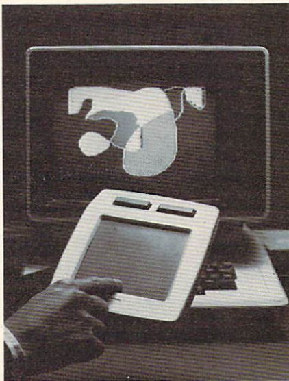
The Koalapad Touch Tablet can be used for drawing or as an auxiliary keyboard.
