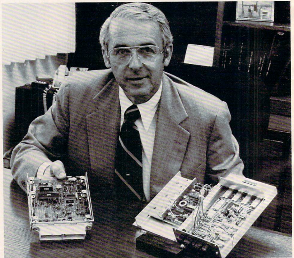
Jerome G. Rivard, chief engineer for Ford's Electrical/Electronics Division, compares the size of the company's original Electronic Engine Control (right) with the latest version. The new controller can process a million commands per second.
