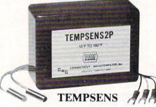
This module provides two temperature probes for use by the AIM16. This module should be used with the MANMOD1 for ease of hookup. The MANMOD1 will support up to 16 probes (eight TEMPSENS modules). Resolution for each probe is 1°F.
