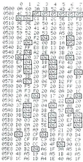
Figure 1b. Monitor in original location, showing bytes to be changed (part 2)
