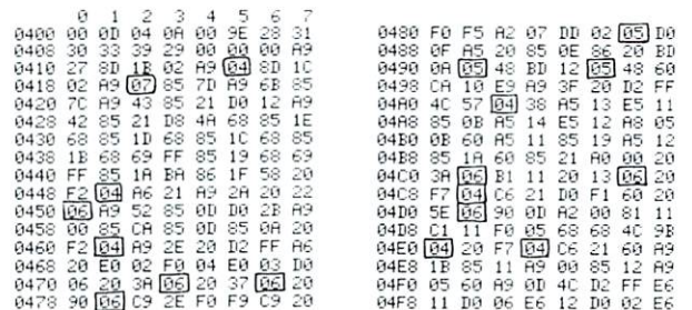
Figure 1a. Monitor in original location, showing bytes to be changed (part1)
