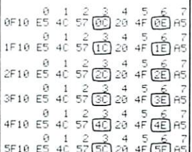
Figure 5. Contents of selected locations after Monitor Multiple Relocator has been run.
