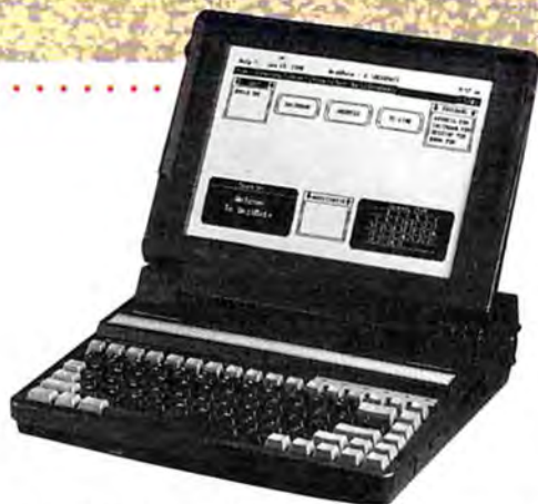
Tandy's 2800 HD puts high-performance computing on the road with one megabyte of memory and a 286 microprocessor in an executive black box.
