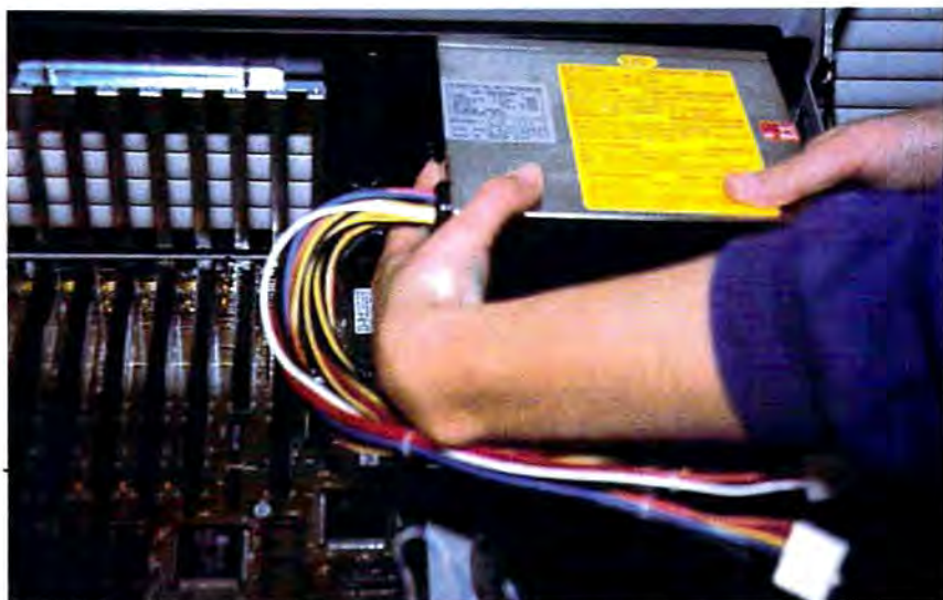
After the motherboard is in place, it's time to install the power supply. Most power supplies slide into position and fasten to the rear of your case.
