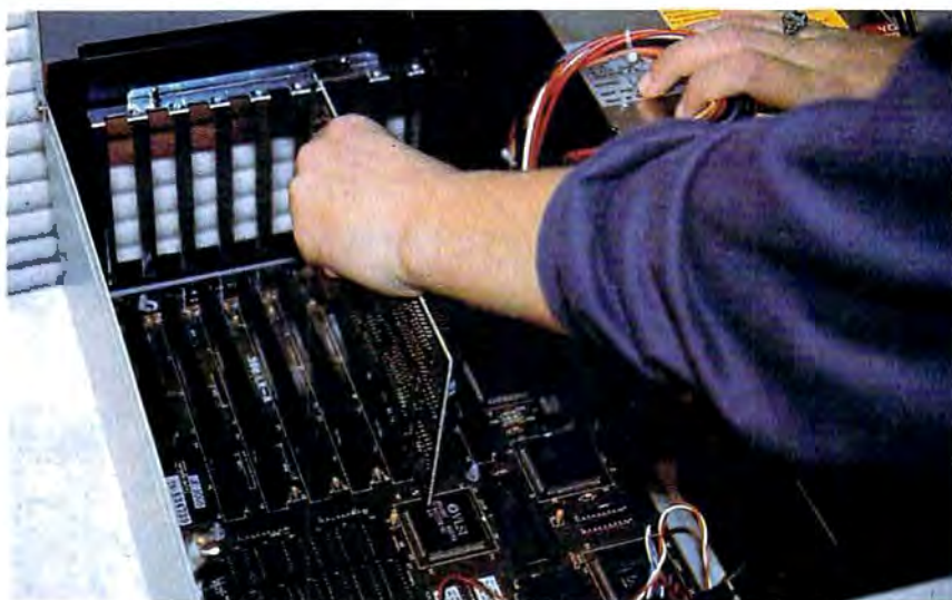
Seat each expansion card by firmly pressing it into its slot; then fasten the the card's back plate to the case.
