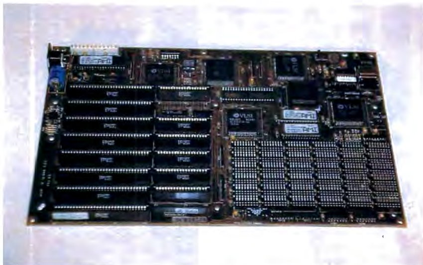
Equipped with AMI BIOS, this motherboard design allows for up to four megabytes of RAM.
