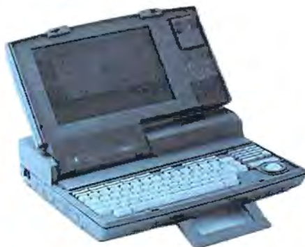
The ST-compatible Stacy laptop from Atari has one megabyte of RAM.
