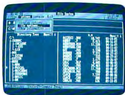
The Shell in DOS 4.0 presents a graphics interface that insulates the user from the command line.
