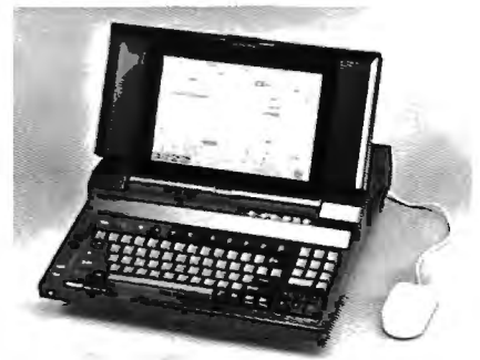
The Yamaha C1 Music Computer orchestrates 11 MIDI ports and a megabyte of memory.
