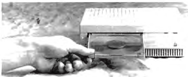
The Apple CD SC downloads from the front using a plastic disc caddy.
