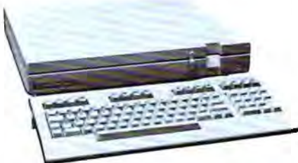
The Commodore 128D features a detachable keyboard and an internal 1571 5¼-inch disk drive.
