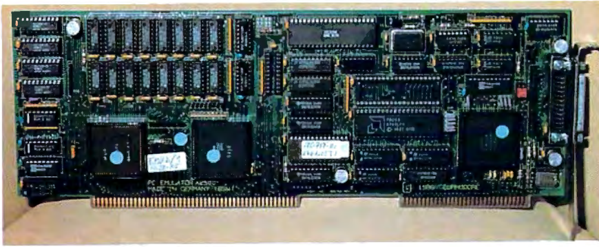
The Amiga Bridge card supplies everything which the Amiga 2000 needs to run IBM PC software, including an Intel 8088 microprocessor, 512K of RAM, and a floppy disk controller for 5¼-inch PC-compatible floppy disk drives. The board can also accept an Intel 8087 math coprocessor.
