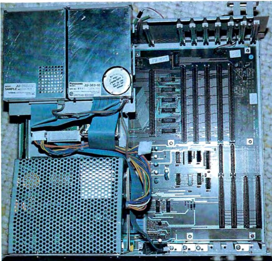
An overhead look at the inside of an Amiga 2000, showing the expansion area to the left and the power supply and internal floppy drives to the right. The bulk of the Amiga's internal circuitry, including its 68000 microprocessor, is not visible from this angle.
