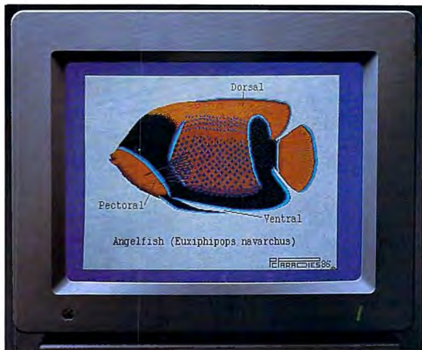
The AppleColor RGB monitor has a 12-inch screen with a resolution of 640 × 200 pixels. When used with the Apple IIGS computer, the monitor is capable of displaying graphics and text in as many as 4096 colors.
