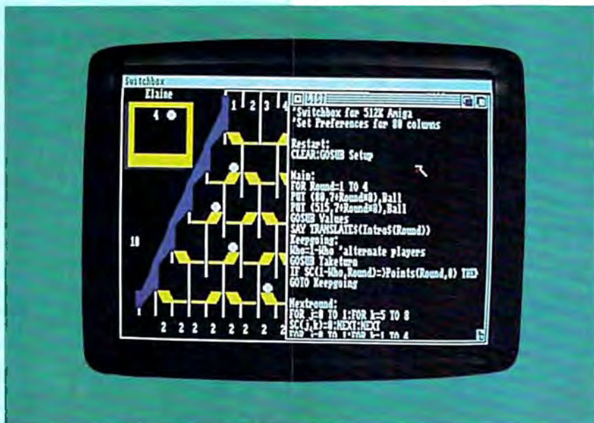
In Amiga BASIC line numbers are unnecessary, and are replaced with labels that indicate subroutines and program divisions.
