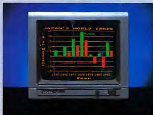
MODEL 420 12 inch Super High-Res RGB Color Monitor. Fully compatible with Apple, IBM and most other personal computers. 640x262 line resolution. Unlimited colors available through analog video circuit. Black face, non-glare tube.
