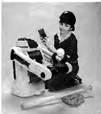
Maxx Steele is a two-foot tall robot with a 150-word vocabulary and 20 preprogrammed phrases. His claw is nearly as flexible as a human wrist.
