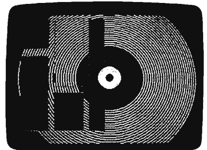
Program 3 shows how concentric circles are automatically scaled only within the small invisible viewport at the center of the screen.
