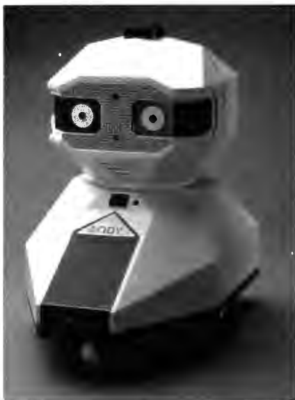
Andy the Personality Robot has a programmable personality and can be controlled with a Commodore 64 or Atari home computer.
